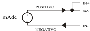
FIG. 4 LOOP 4...20 mA +/- 0...40 mA
